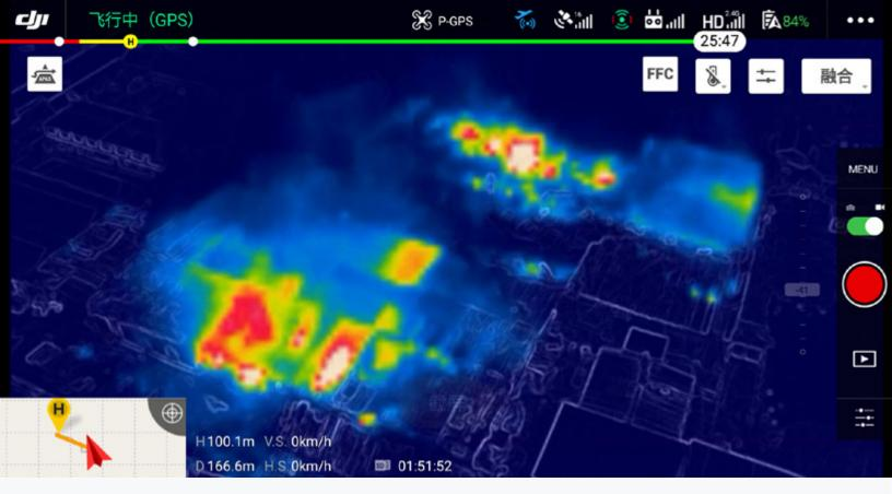
Drone-based thermal imaging can assist in determining which structure quadrants have the hottest heat signatures and what, if any, extensions exist.
